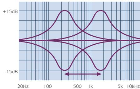
15dB of cut or boost is available at low, mid and high frequencies, giving plenty of control just where it's needed
