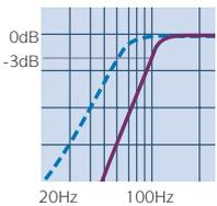
a dashed line in the diagram) which means that all of the lower frequencies are attenuated – a less steep slope allows more bass
