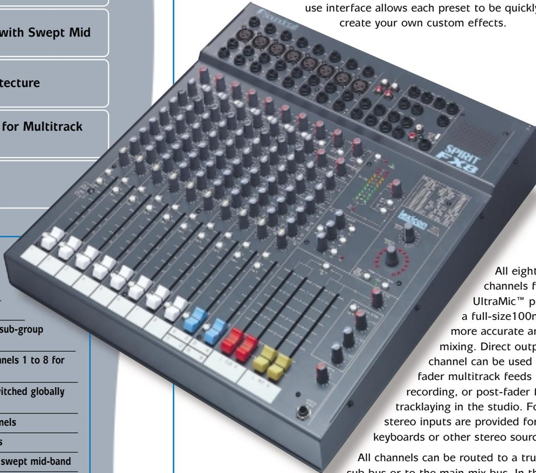
All eight mono channels feature an UltraMic™ pre-amp, plus a full-size 100mm fader for more accurate and precise mixing. Direct outputs on each channel can be used either as pre-fader multitrack feeds for live recording, or post-fader feeds for tracklaying in the studio. Four pairs of stereo inputs are provided for effects, keyboards or other stereo sources.
