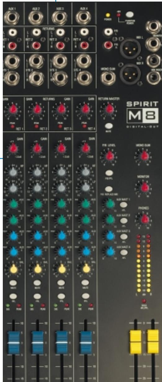
fade signal is fed to the headphones, control room output and meters, with levels displayed on the left and right meters in mono to enable levels to be monitored without interruption to the main mix.
